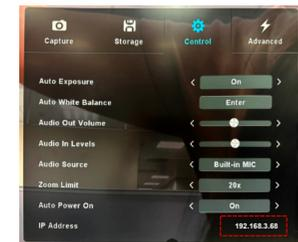
PS753 DHCP is enabled by default. You can use remote control to open **Menu > Setting > Control** to check the IP address. Open the browser, and enter the IP address in the address bar.
